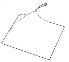
Figure 5. Removing Adhesive Backing
